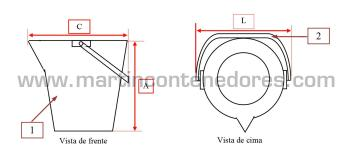
$C*L*A \Rightarrow 260*257*233mm$  $\varnothing$  interior do bordo superior  $\Rightarrow 210mm$
